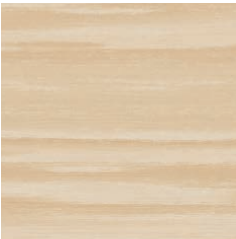
TM002 12mm thk Marine Plywood Dimension: As specified on drawings. Finish: To match interiors (unless specified otherwise)
